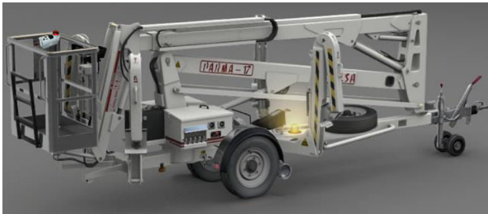
A Parma 17 unit with most accessories including Galvanized Iron Basket & Articulated Hydraulic Stabilizer
